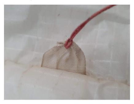
We conducted a breaking test study on the line/attachment tab mounting with a static (sustained) and dynamic (shock) load to see the influence of the mounting method to the overall strength.
