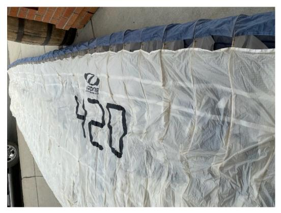
Despite 3 seasons of flying and having spent 25 days exposed in the desert, the cloth is still in relatively good condition. The average lower surface porosity reading is 73 seconds with a tear strength of 1000g (5mm tear measured with a Bettsometer). The upper surface leading edge has an average porosity of 239s and a similar tear strength of 1000g.
