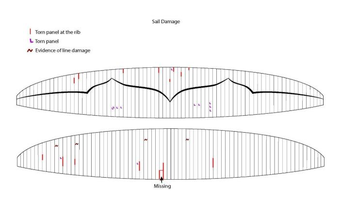
A few lower surface panels exhibit evidence of serrated tears caused by line damage, identifiable by the red marks left by the lines in the area of the tear. These marks are typical evidence of line failures after extremely high loads and are caused by the whiplash effect of the broken lines. We regularly observe exactly the same type of damage on wings that have been subjected to a destructive load tested. See photos below:
