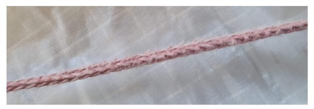
This type of damage indicates a strong possibility of a "twisted line" incident. Broken fibres and discolouration caused by excessive frictional forces during a twisted spiral can significantly reduce the strength of individual lines.
